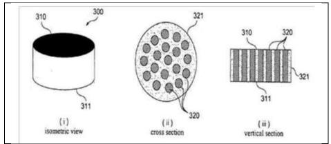
Fig. 3: Schematic Diagram of Innowattech Piezo lectric Generator.
