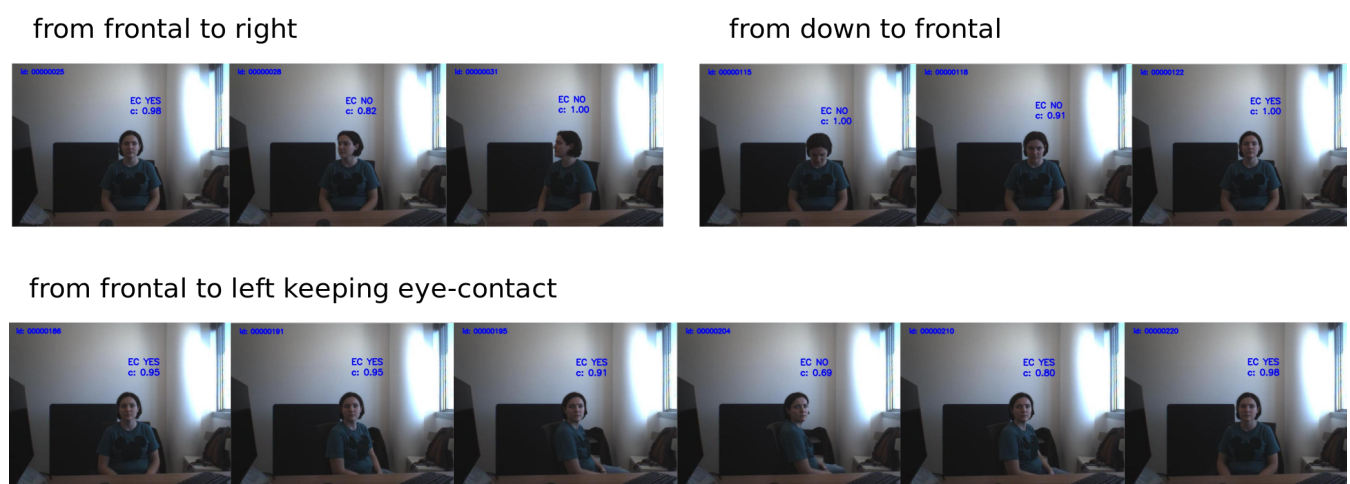
Figure S4. Transition scenarios. Three sequences of frames representing different transition scenarios: from frontal to right, from down to frontal and from frontal to left keeping eye-contact with iCub. The prediction with the confidence score are in blue on each single frame.
