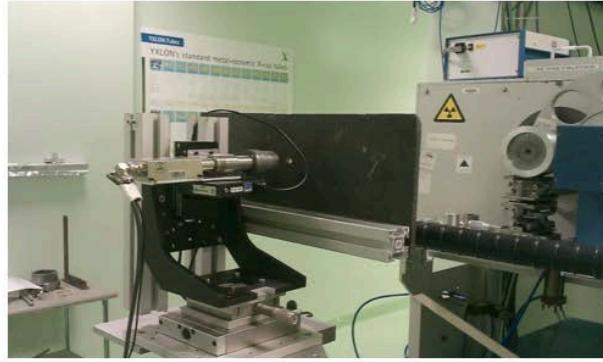
211 212 213 Figure 1. Schematic representation of the spectrometer positioning in the X-ray field (left), and the 214 experimental set-up used for the X-ray spectra measurements, emitted by the CEA X-ray generator (right).
