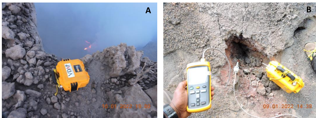
Figure 11. MultiGas deployment at the summit of Mt Nyiragongo (A) and the eruptive site of May 2021 near Kibati
