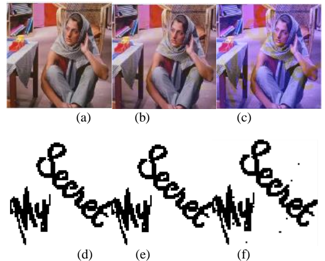
Fig. 5. Watermarked image of Barbara : (a) \alpha = 5 , (b) \alpha = 20 , (c) \alpha = 80 . Secret/watermark image: (d) extracted from (a), (e) extracted from (b), (f) extracted from (c)
