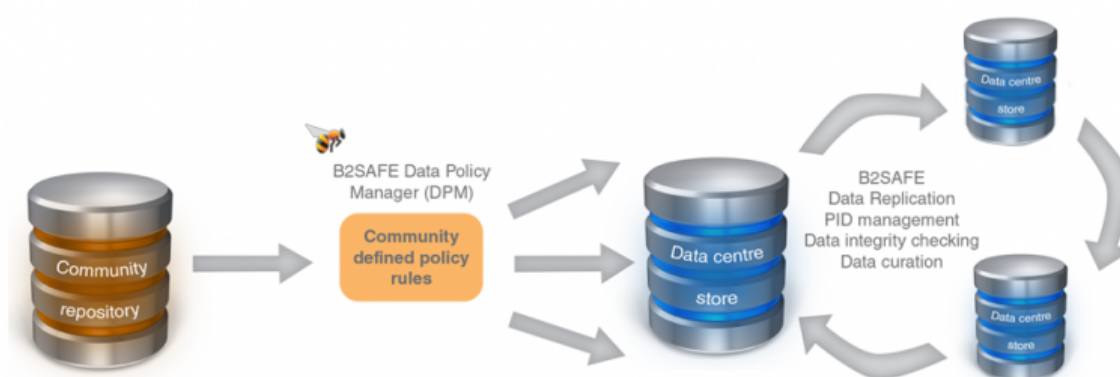
Figure 3: B2SAFE Process & Architecture
