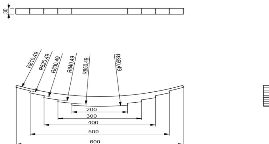
**Figure 1.** Diagram of composite leaf spring
