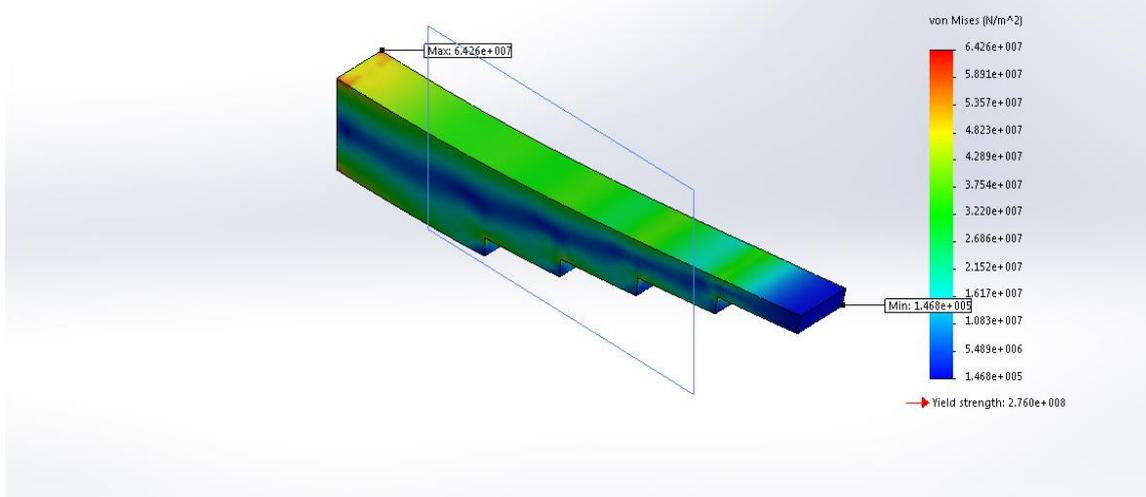
**Figure 3.** Von misses stress of Carbon fiber leaf spring
