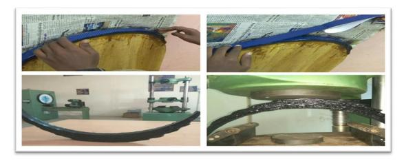
Figure 2. Fabrication details
