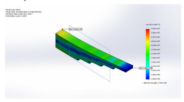
Figure 3. Von misses stress of Carbon fiber leaf spring
