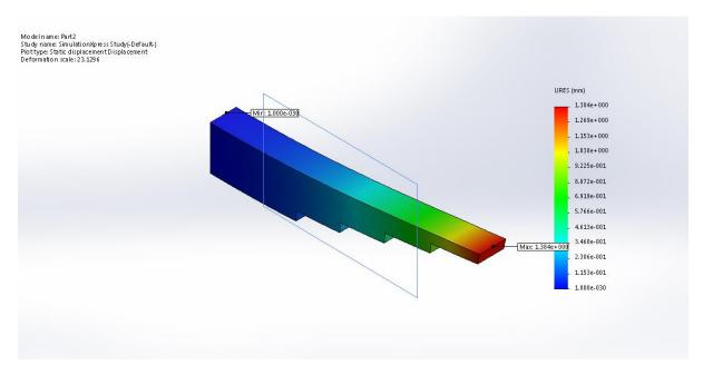
Figure 4. Deflection test for carbon fiber leaf spring
