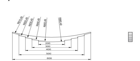
Figure 1. Diagram of composite leaf spring
