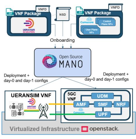
Figure 5-4: High-level workflow of manual deployment of a 5G network.
