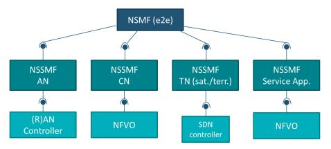
Figure 5-2: Architectural diagram of Network Slice Management in 5G network.
