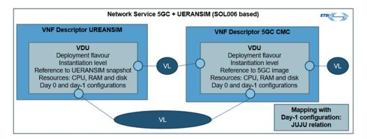
Figure 5-5: High-level diagram of Network Service
