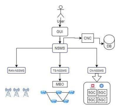
Figure 3-2: 3GPP architecture 28.531 to create end to end slice resources.
