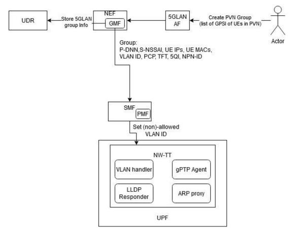
Figure 2-1: UPF architecture with modules to implement 5GLAN functionality.
