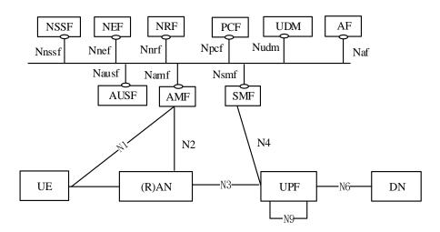
Figure 1-2: 5G Service Based Architecture.
