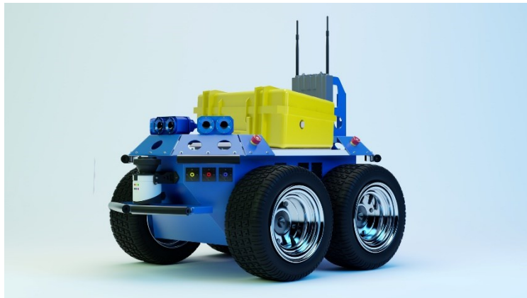
Figure 18: RESCUE-MIMS on-board DFKI robotic platform SeekurJr
