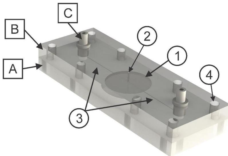
**Fig. 1.** Chip: A - bottom part; B - top part; C - tube fitting; 1 - main chamber; 2 - air pillar, for removing bubbles; 3 - supply channels
