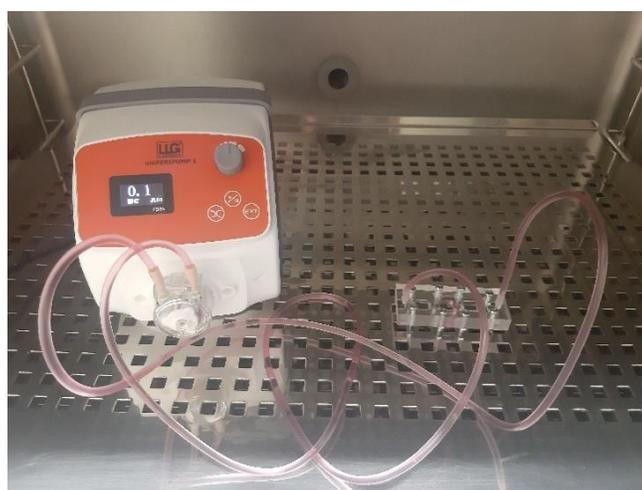
**Fig. 7.** Chip connected to a peristaltic pump with flow
