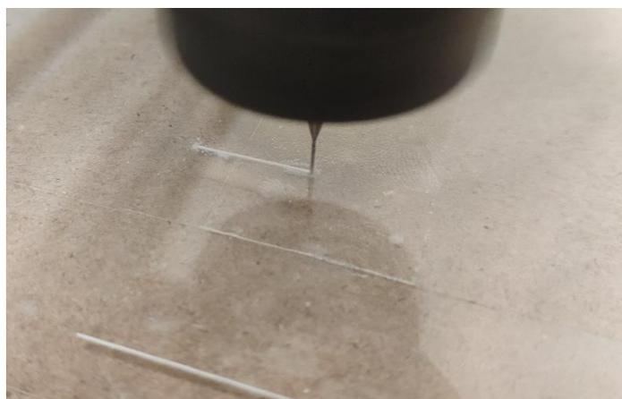
**Fig. 5.** Milling process, ball end flute 0.25 mm
