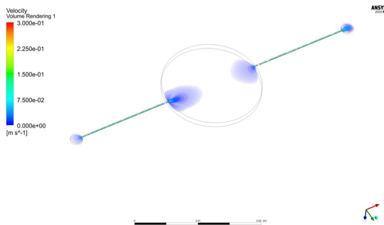
**Fig. 2.** Fluid velocity — PAK solver, input fluid velocity 0,03 ml/s.
