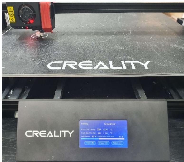
**Fig. 6.**3D printing of tubing fittings
