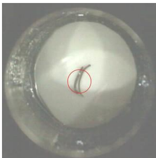
Fig. 7 Samples from project Plast- Morgondagens kulturobjekt , small pieces on the measuring window with a red circle marking the area of analysis of 4 mm diameter, SurveNIR camera.
