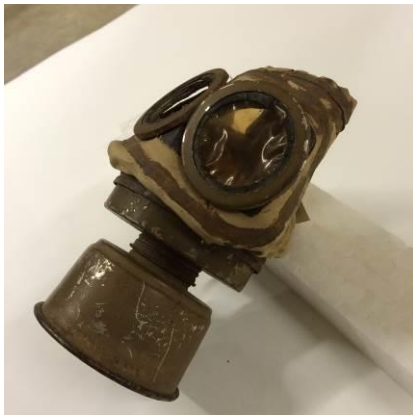
Fig. 15. Gas mask from Verdun WW1 with eye pieces made of semi-synthetic cellulose.
