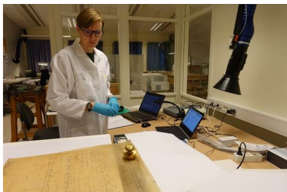
Fig 16. SurveNIR instrument set up at the Swedish National Archives Arninge investigating construction drawing.
