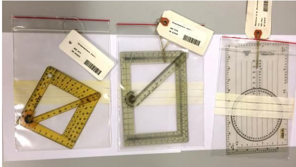
Fig 13. Measuring rulers made of cellulose nitrate, cellulose acetate and polystyrene.
