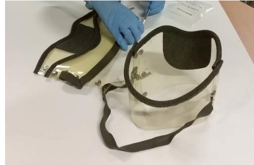
Fig. 14. Motorcycling wind shields made of cellulose nitrate (or cellulose acetate in one case only).
