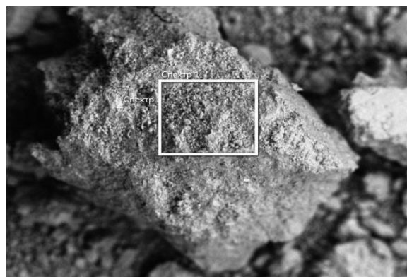
Figure 1. a) Spectrogram of bentonite clay b) Photograph of grain bentonite clay enlarged 250 times,
