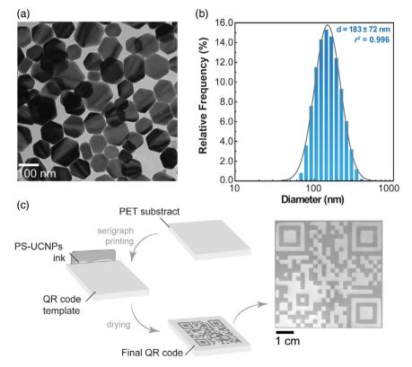
**Figure 2.** a) TEM images and b) hydrodynamic size distribution of the NaGdF<sub>4</sub>:Yb<sup>3+</sup>/Er<sup>3+</sup> UCNPs. The gray line is the best fit to the DLS data using a lognormal distribution ( $r^2 = 0.996$  and fitting parameters shown in Table S1, Supporting Information). c) Schematic representation of the preparation of the QR codes and the final QR code (encoding the URL http://iq.unesp.br) under white light illumination.
