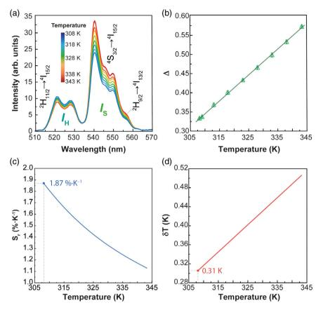
**Figure 3.** a) Temperature-dependent upconversion emission spectra of the QR codes in the 308–343 K range measured at  $P_D = 40 \text{ W cm}^{-2}$ . b)  $\Delta(T)$  calibration curve. The solid line is the best fit to the data using a straight line ( $r^2 > 0.99$ , fitted parameters are shown in Table S2, Supporting Information). c) Relative thermal sensitivity and d) temperature uncertainty of the QR code luminescent thermometer.
