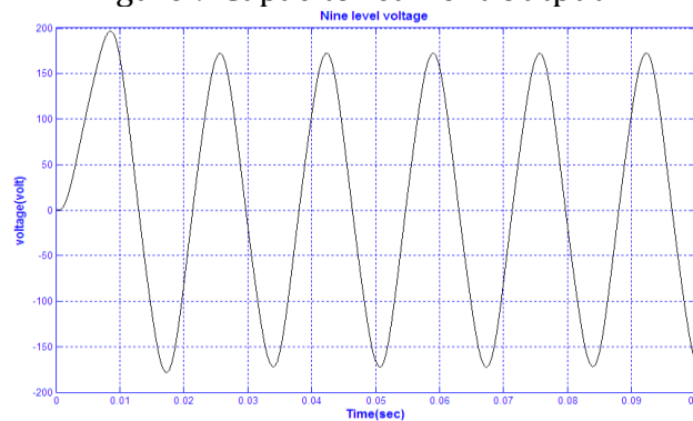
Figure 10: Nine level Voltage Output
