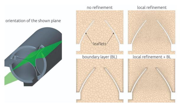
Figure 2: Visualization of different mesh refinement strategies for a finite volume mesh of a biological valve prosthesis within a tube. The geometry to be meshed is shown in the left panel together with a plane (green) in which the mesh is visualized. The right panel shows four different polyhedral meshes using local refinement at the leaflets, boundary layers at all surfaces, a combination of both approaches as well as a baseline mesh without refinement.
