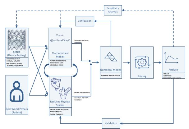
Figure 1: Exemplary simulation workflow to provide an overview of the following simulation steps: physical problem, modelling, running the simulation, and analysing the results.
