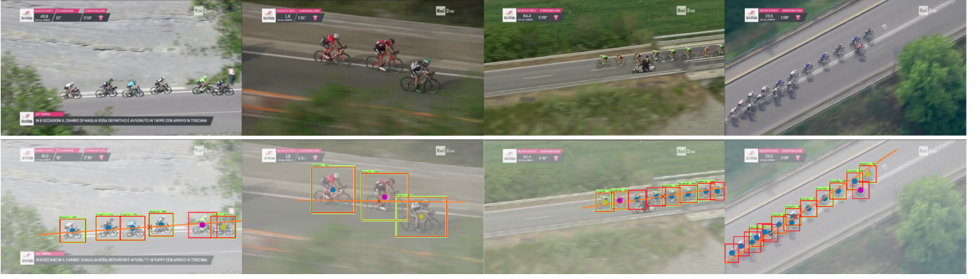
Fig. 3: Cyclist ranking. The first row shows the source video frames and the second row shows the processed ones. The orange line indicates the estimated target motion direction. The yellow, magenta and blue dots stand for a) the leader, b) the second best and c) the rest of the ranked targets respectively.
