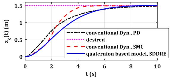
Fig. 4.  $z$ -axis regulation of the system, comparison with PD and SMC.
