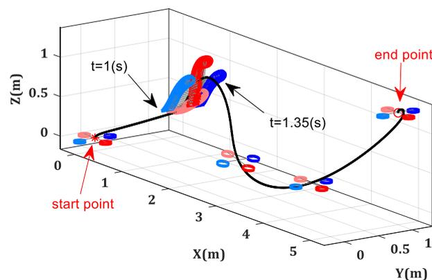
Fig. 12. The Cobra maneuver via the SDDRE and quaternion dynamics.
