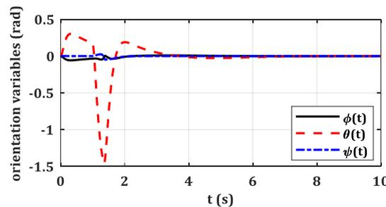
Fig. 11. The Euler angles of the drone in aerobatic maneuver.
