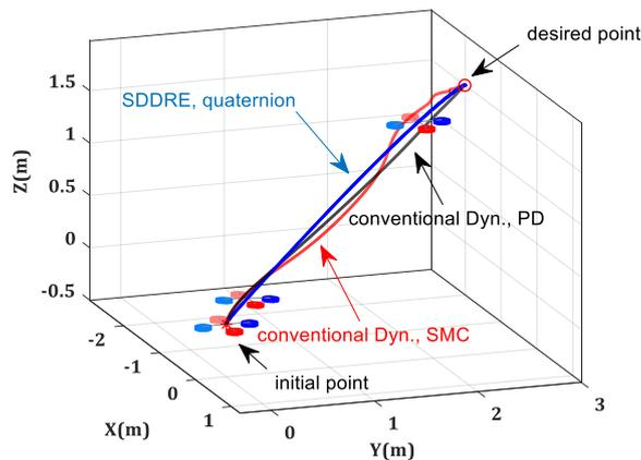
**Fig. 8.** The configuration and trajectories of the quadrotor drones with PD, SMC, and SDDRE controllers.
