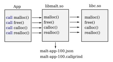
Figure 1 MALT intercepts allocation calls using Linux's LD\_PRELOAD. [1]
