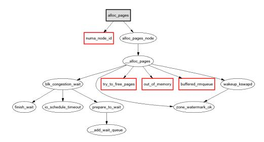
Figure 13 A sample Call graph of alloc\_pages() in the Linux Kernel 2.6.12-rc2 made using CodeViz [2]
