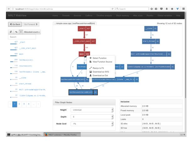
Figure 22 The completed Call Tree page. Notice the filter controls at the bottom and the Symbol List on the left-hand side. The context menu is also open in this particular screenshot.
