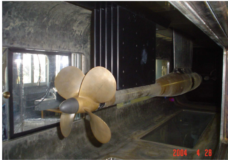
Figure 12: Tunnel set-up with propeller and wake generator.
