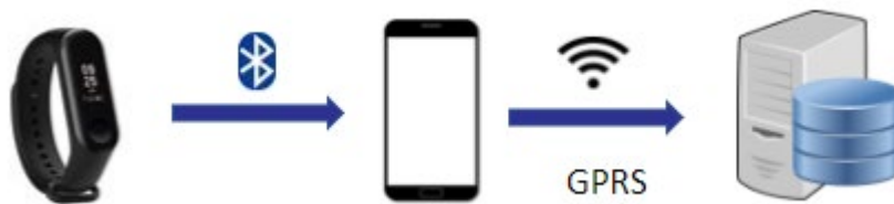
Figure 6.8.1 Sensor data generation and communication
