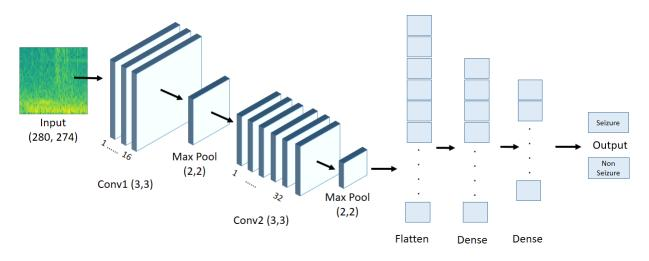
Fig. 2. Generic CNN Pipeline for seizure detection using Rhythmicity Spectrogram.
