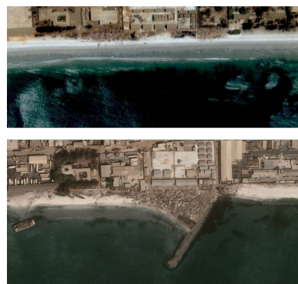
Figure 7. Thiaroye Sur-Mer. The construction of a breakwater leads to an accretion zone that has been urbanised. Source: Google Earth.
