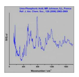
Inelastic Neutron Scattering spectrum of Urea/Phosphoric Acid, NH<sub>2</sub>CONH<sub>2</sub>/H<sub>3</sub>PO<sub>4</sub> measured on the TOSCA instrument
