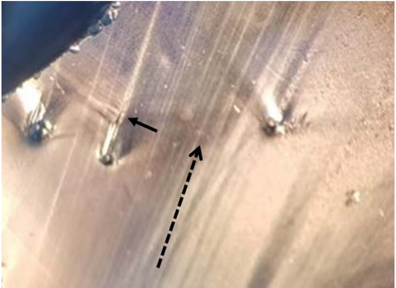
Figure 4.13: Wake hackle in glass; solid arrow points to a wake hackle line and the dashed arrow indicates the direction of crack propagation
