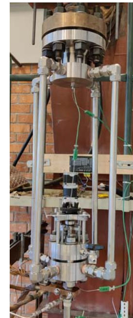
Multisensor probe unit of the HWAT facility (KTH) →
