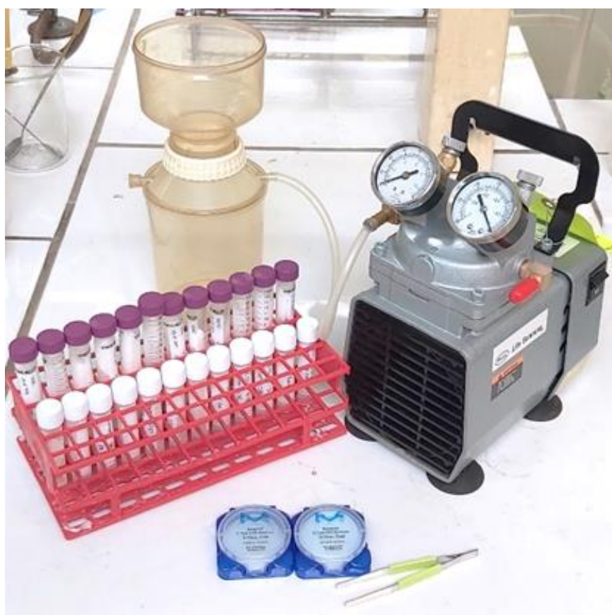
Fig.4.2 | Vacuum pump and filtration apparatus for eukaryotic plankton sampling >0.22 \mu\text{m} and filter containers (cryotubes)
