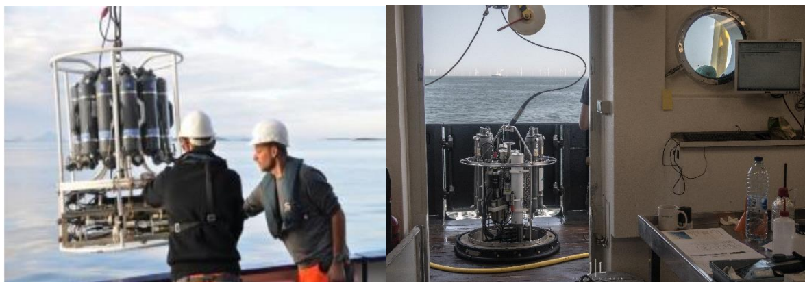
Fig. 4.1 | Left: Sea-bird SBE25 (on board RV Simon Stevin). Right: Sea-bird SBE911 CTD probe (on board RV Heincke).
