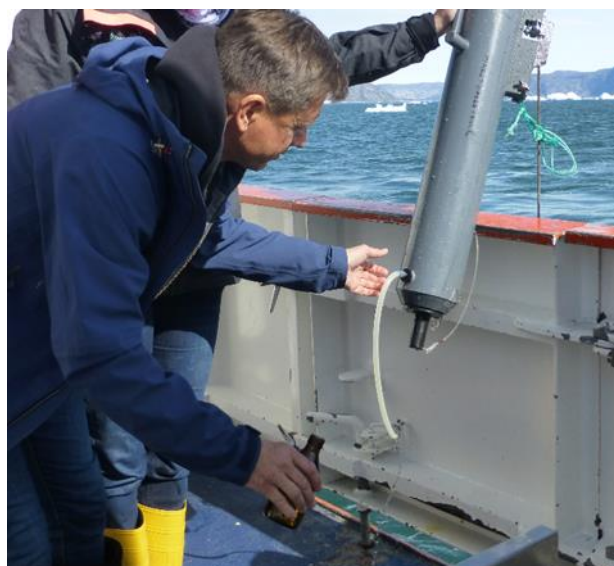
Fig. 5.2 | Silicon tube used to reduce organism loss when water samples are collected with Niskin bottles.
