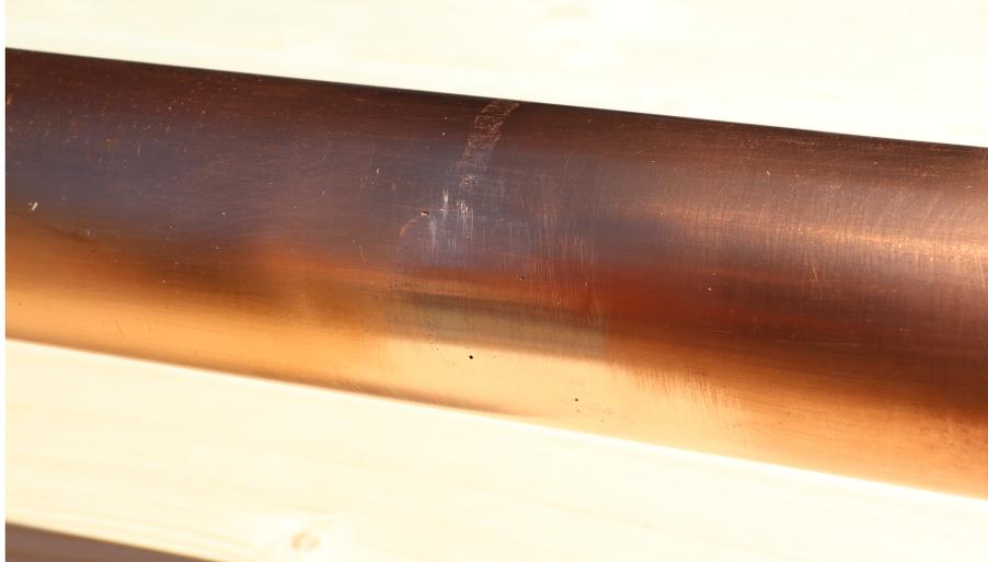
**Figure 4.6:** Region around the welding seam for the copper reference tube. Several defects in and a rather rough surface are visible.
