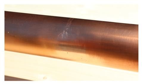
**Figure 4.6:** Region around the welding seam for the copper reference tube. Several defects in and a rather rough surface are visible.
