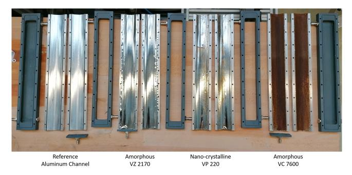
Figure 4.12: Dissembled experimental heat exchanger after long term water exposure
