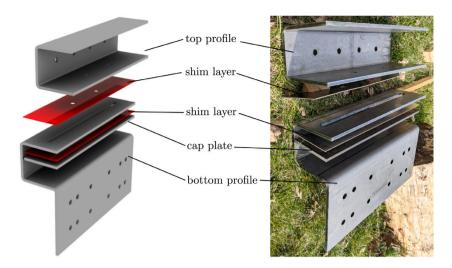
Fig. 5. Illustration and photographs of the parts of the specimen.
