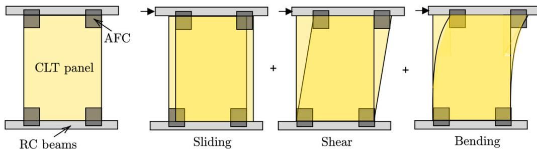
Fig. 10. Qualitative explanation of CLT panel response.
