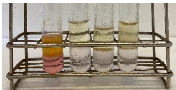
FIGURE 5: Colouring of the reference sample compared to those from the Ca (II) / Cu (II) cation exchange
