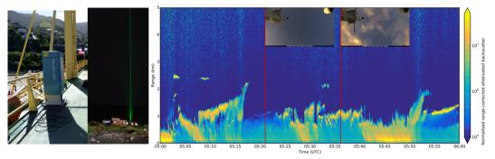
Simulated spaceborne lidar, 532 nm wavelength
