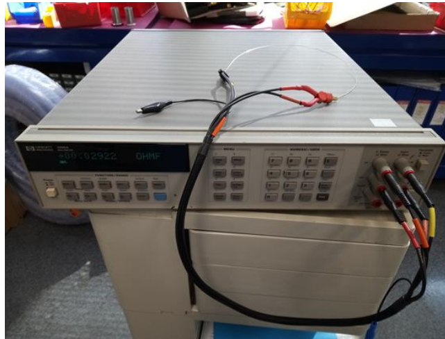
Figure 6. RRR measurement: room temperature setup.
