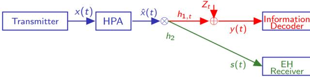
Fig. 1. A SWIPT system over a fading channel with HPA at the transmitter and a non linear EH channel.
