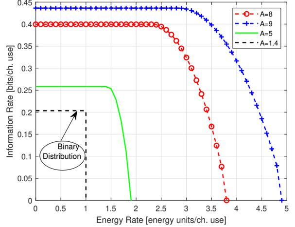
Fig. 2. Information-energy capacity region with different PP constraints;  $\beta = 1$ ,  $P = 30$  dB.
