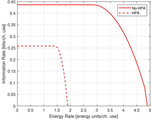
Fig. 3. Effect of the HPA on the Information-energy capacity region;  $A = 5$ ,  $\beta = 1$ ,  $B = 0.5$ ,  $P = 30$  dB.
