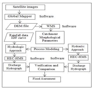
Fig. 2 The developed GIS-based flood assessment methodology.
