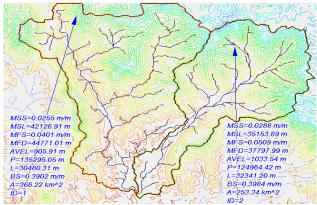
Fig.5. Basins Delineation and their morphological characteristics with the aid of WMS
