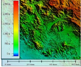
Fig. 3. DEM Model for Adam Area extracted from **GlobalMapper**®
