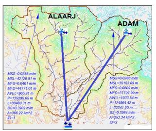
Fig. 6. Schematic simulation of the catchment area representing Outlet Point and catchment area sub-basins
