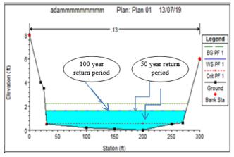
Fig.8. HEC-RAS output showing wadi's typical cross-section at Alsahwah, Adam.
