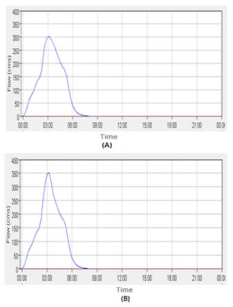
Fig.7. Discharge Hydrograph at outlet created by HEC-HMS for (a)50- yr and (b)100-yr Return period.
