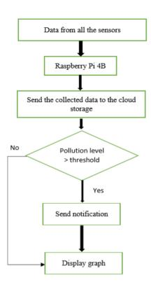
Fig. 8. Flow of data within the system.
