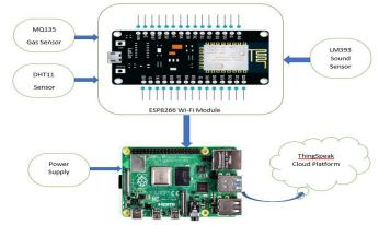
Fig. 6. System Architecture.
