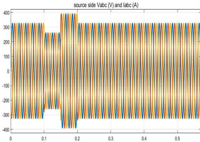
**Fig:4.5 Phase A,B&C supply voltage and current without DSTATCOM [before voltage compensation]**
