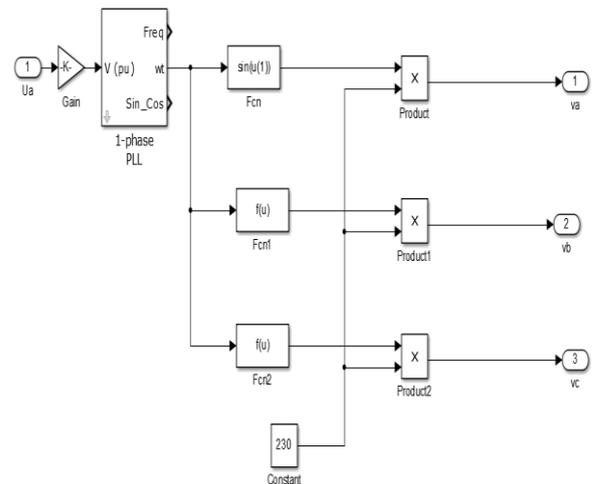
Fig: 4.3 Reference voltage generation
