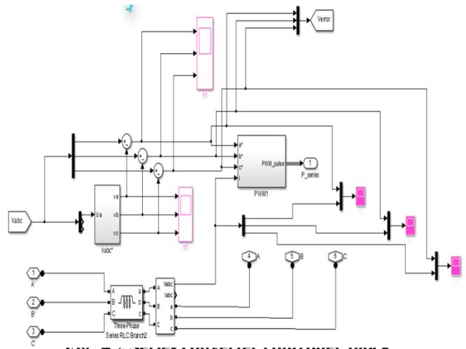
Fig. 4.2 Series Converter Controller Block
