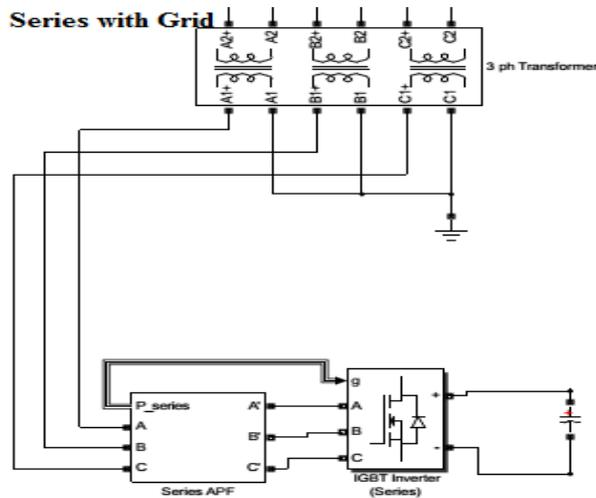
Fig: 4.1 Voltage Compensation block.
