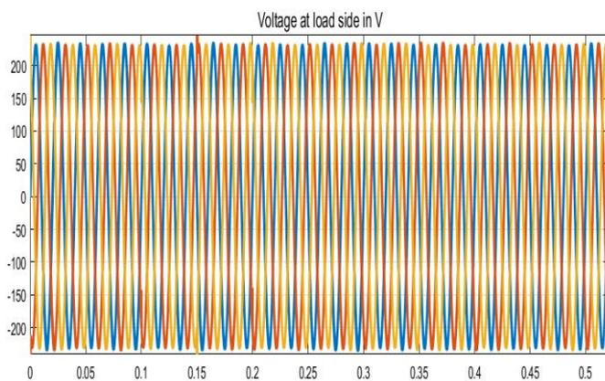
**Fig:4.6 Phase A,B&C Load voltage with DSTATCOM [after voltage compensation]**
