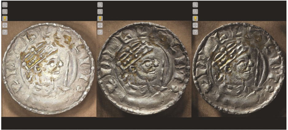
Fig. 18. An example of an online RTI viewer, using three different positions of the light source. Source: Pickup Ch., William II Coin Obverse RTI Demo, Institute of Information Science and Technologies "Alessandro Faedo", downloaded from https://s3-eu-west-1.amazonaws.com/cp-rti/Anja-Coin.HTML , accessed December 2021.
