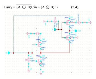
Fig. 2 Schematic diagram of 4T XOR logic circuit
