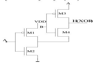
Fig.14T XOR logic circuit
