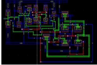
Fig.9(a) Layout of N17T adder
