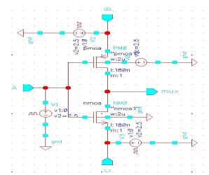
Fig. 3 Schematic diagram of 2T MUX logic circuit
