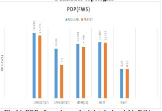
Fig.16. PDP of regular and triplet design 4-bit RCA Fulladdertopologies
