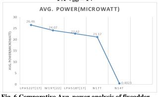
Fig. 6 Comparative Avg. power analysis of fiveadder topologies
