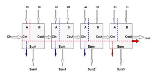
Fig. 11 4-bit RCA regular design [17]
