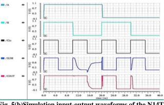
Fig. 5(b)Simulation input-output waveforms of the N14T FA  $V_{DD} = 1V$
