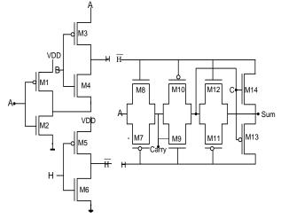
Fig. 4(b) N14T FA circuit
