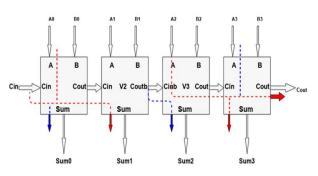
Fig. 124-bit RCA triplet design [17].
