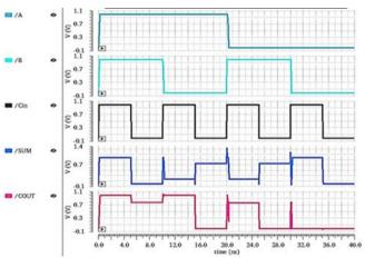
Fig. 5(a)Simulation input-output waveforms of the N17T FA  $V_{DD}$  = 1V
