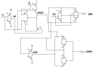
Fig. 4(a) N17T FA circuit
