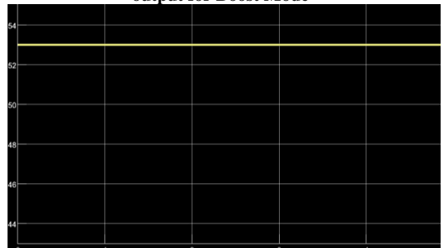
Figure.3 (b). Simulation result for 24V input to 53V dc output for Boost Mode
