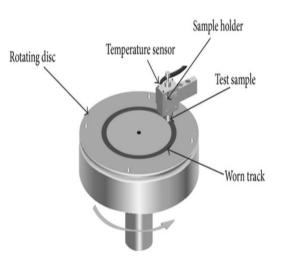
Fig. 1: Pin-on - Disk schematic diagram
