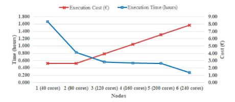
Fig. 3: Execution Time (hours) and Execution Cost (€) vs Nodes
