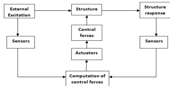
Fig. 1. Flow chart of active control system
