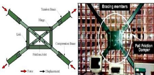
Fig. 5. Friction damper
