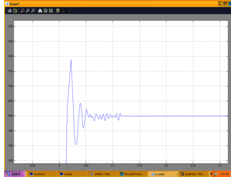
Fig.6.b.Fuzzy controller response for Sawtooth Noise Disturbances (Speed of DC Drive(rpm) Vs time(ms))
