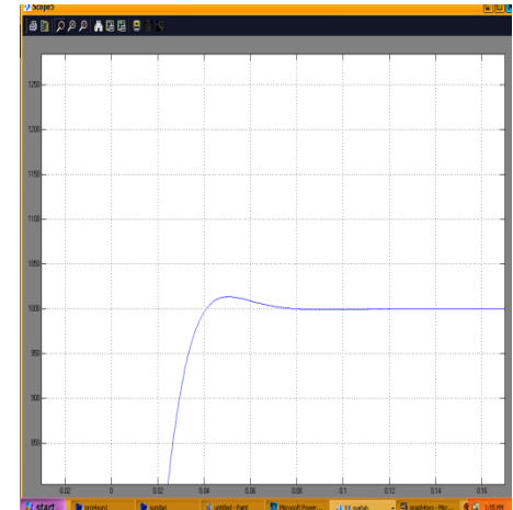
Fig.5.b. GA-PID controller response for Sawtooth Noise Disturbances (Speed of DC Drive(rpm) Vs time(ms) )
