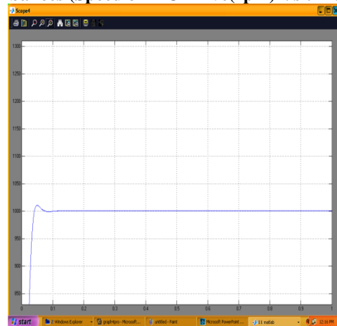
Fig.5.c. GA-PID controller response for Ramp Noise Disturbances (Speed of DC Drive(rpm) Vs time(ms) )
