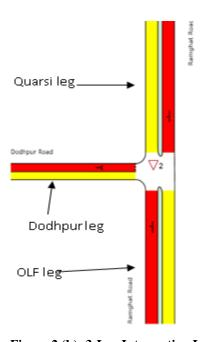
**Figure 2 (b): 3-Leg Intersection Layout in SIDRA** Numerous studies have taken capacity, LOS, delay (geometric and control), travel speed into consideration to quantify the operational performance and efficiency of the intersections [13-20]. To simulate and analyze with efficacy and to be compliant with previous studies, we also have taken these traffic flow parameters as the performance
