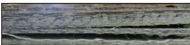
Figure 11: Delamination between Layers in Bamboo Laminated Composites [17-18].
