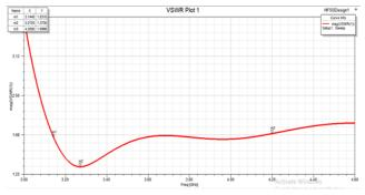
Fig.8 VSWR plot of the designed MIMO antenna
