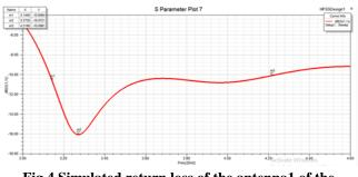
Fig.4 Simulated return loss of the antenna1 of the Proposed MIMO antenna (S1, 1)
