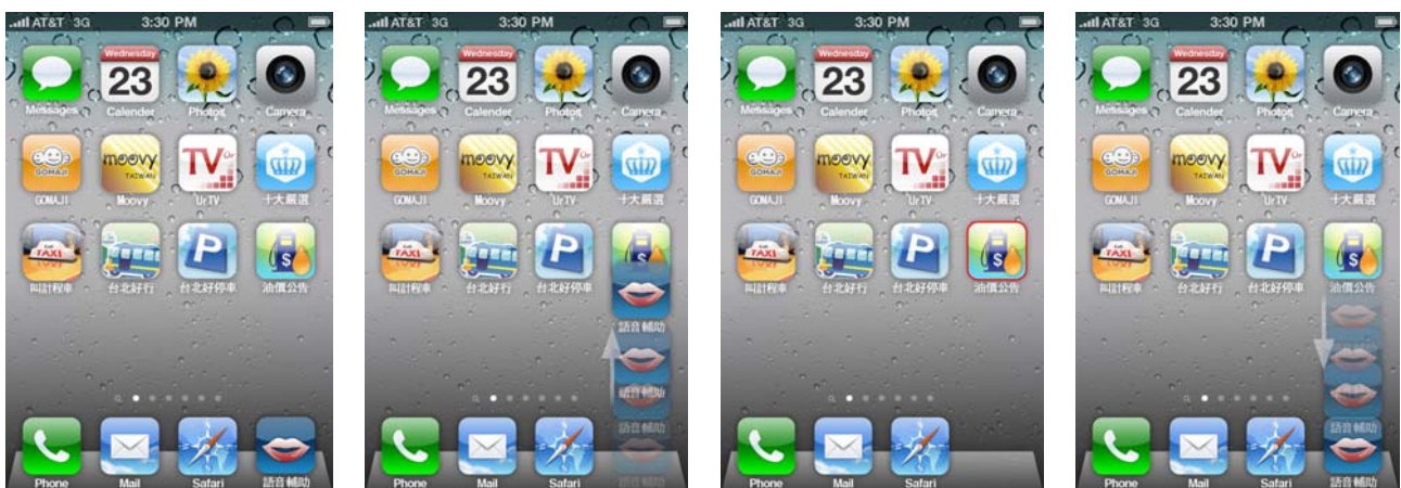
Figure 2. The graphic audio switch was aligned with basic function iconic keys at the bottom of touchscreen.
