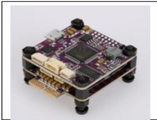
**Figure: Flight Controller**
